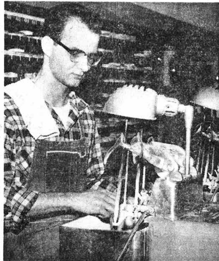
Its final polish is given to a lens in an operation similar to the whetting of a knife blade. The cylinder polishing machine is operated by Donald K. Flanagan. (Piedmont photos)
